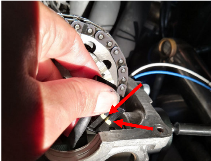
Figure 11 - Slide the Sensor Spacer In
