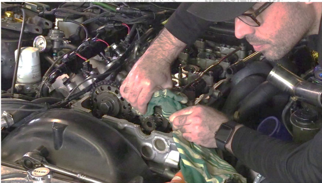
Figure 4 - Remove the Exhaust Cam Sprocket Bolt
