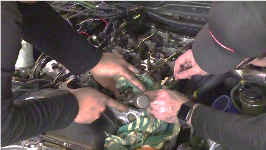
Figure 5 - Removing the CAS Gear
