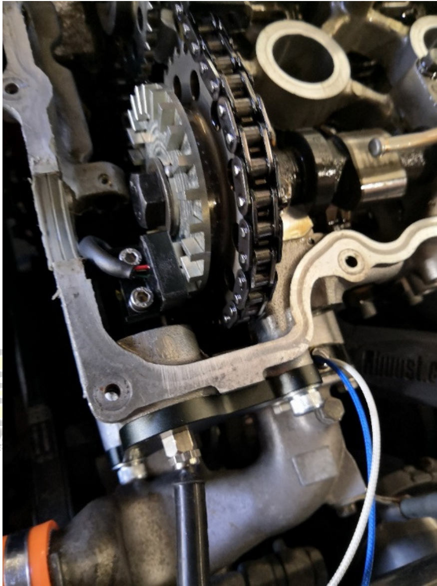
Figure 13 - Installation of the Cam Trigger Kit is Now Complete
