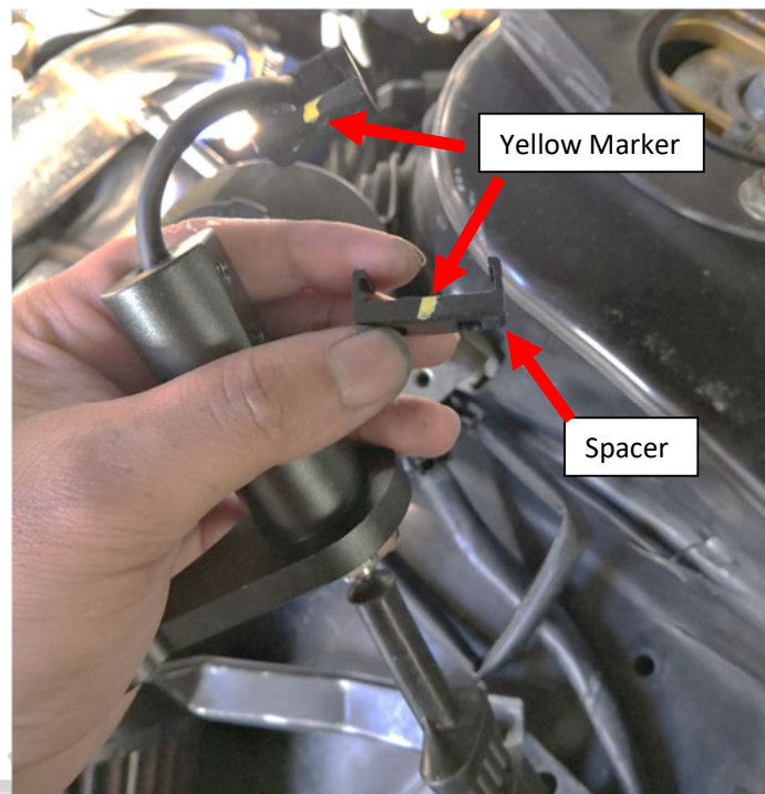
Figure 9 - Cam Sensor and Mounting
