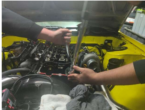
Figure 11 – Torque Cam Bolt to Spec
