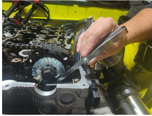
Figure 10 – Check Sensor Air Gap
