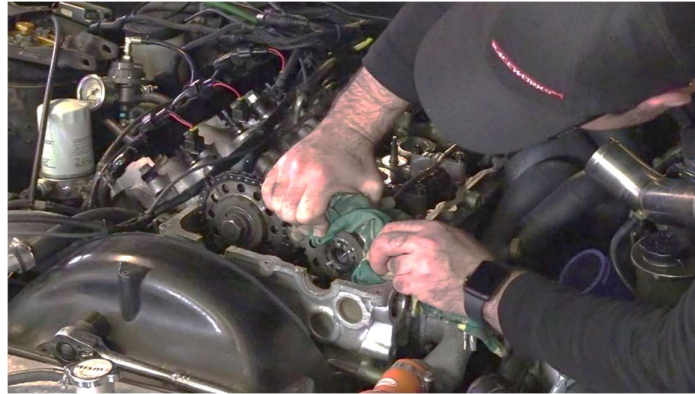
Figure 5 - CAS Gear Removed, 2nd Person Holding the Sprocket Firmly
