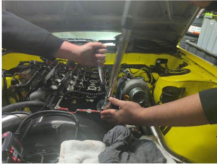
Figure 10 – Torque Cam Bolt To Spec
