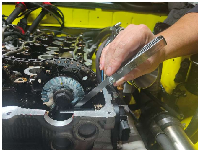
Figure 9 – Check Sensor Air Gap
