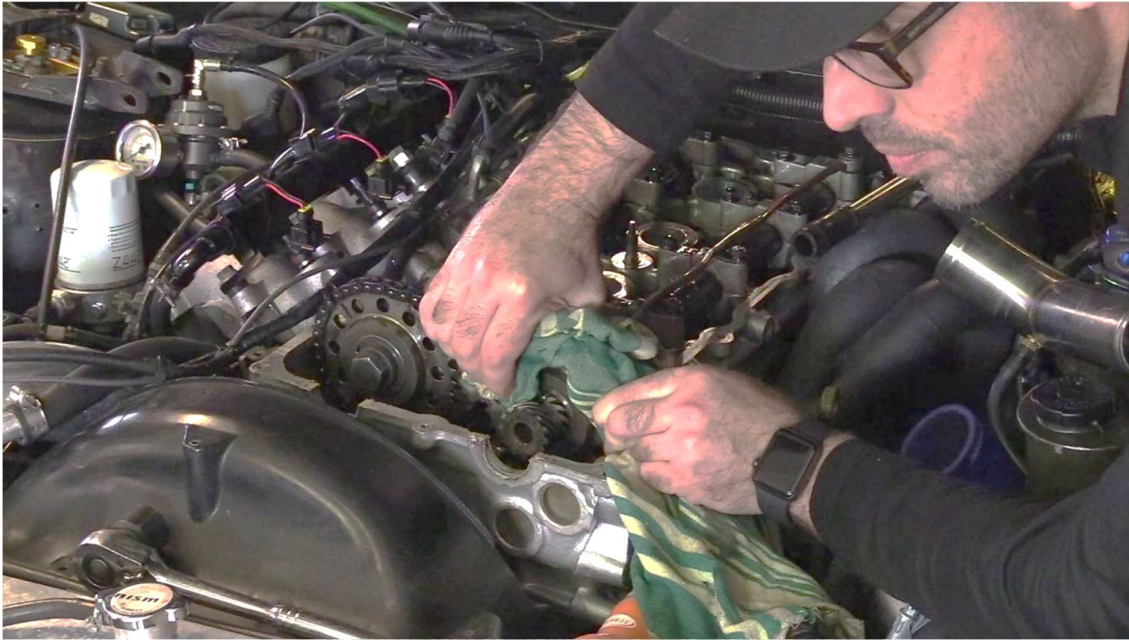
Figure 3 - Remove the Exhaust Cam Sprocket Bolt
