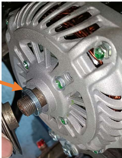
Figure 7 - Install the supplied pulley spacer for short OEM pulley
