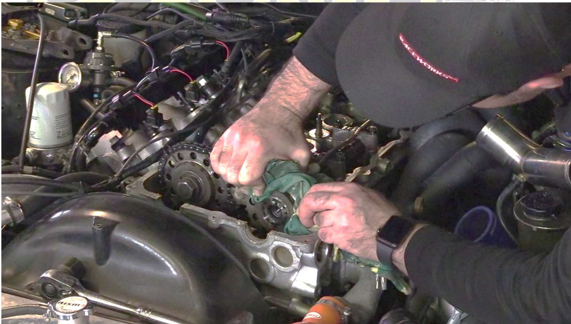
Figure 6 - CAS Gear Removed, 2nd Person Holding the Sprocket Firmly
