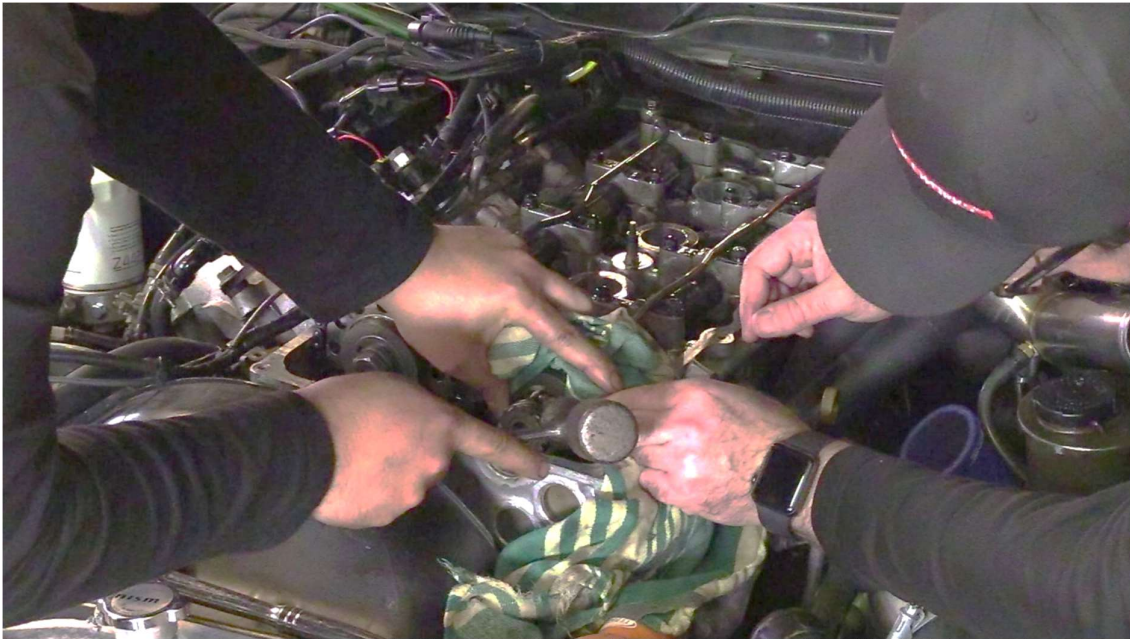
Figure 5 - Remove the CAS Gear
