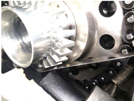
Figure 12 – Checking the Sensor Gap IS MANDATORY!
