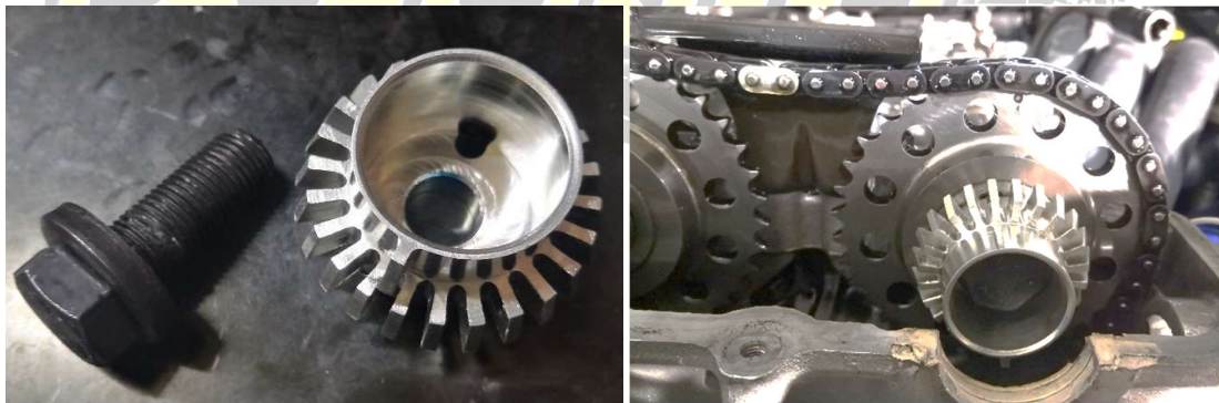
Figure 8 - Trigger Wheel Installed
