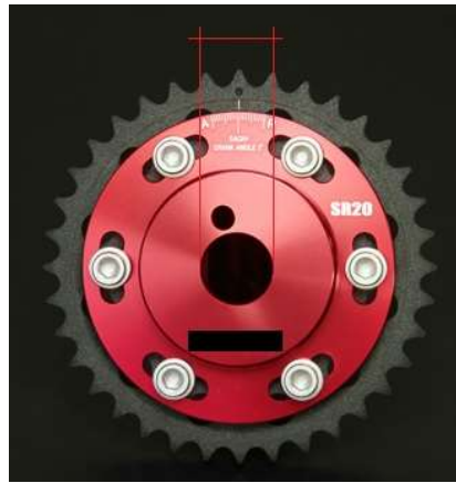
Figure 7 - Measure the internal diameter of the cam gear hub
