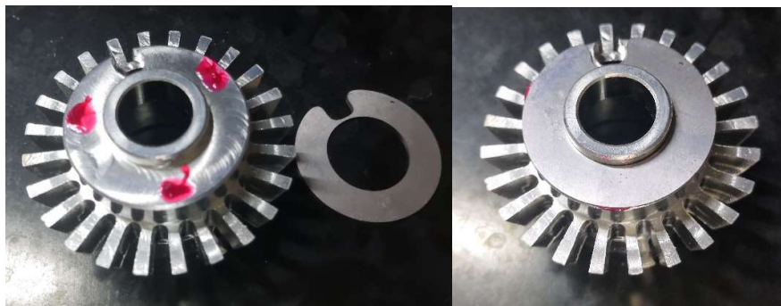
Figure 9 - Install Shim onto Trigger Wheel to reduce the Gap ONLY IF REQUIRED .
