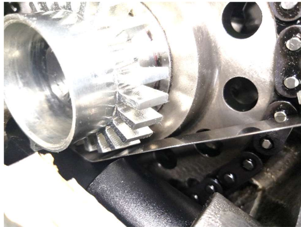
Figure 12 – Checking the Sensor Gap IS MANDATORY!
