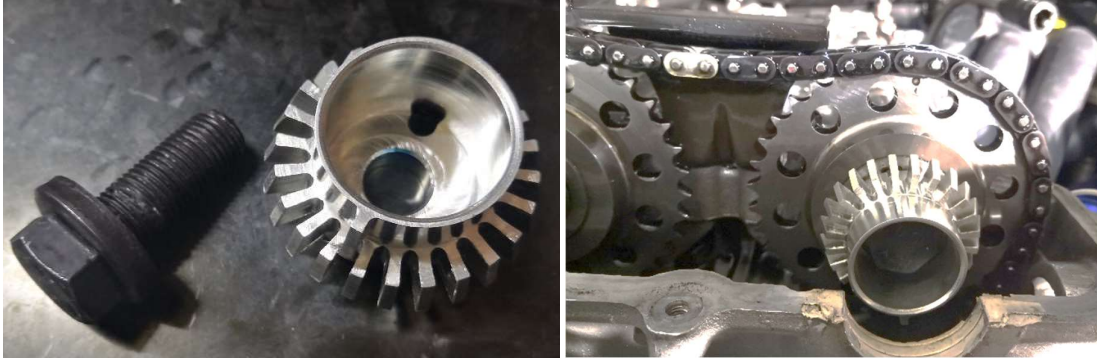
Figure 7 - Trigger Wheel Installed
