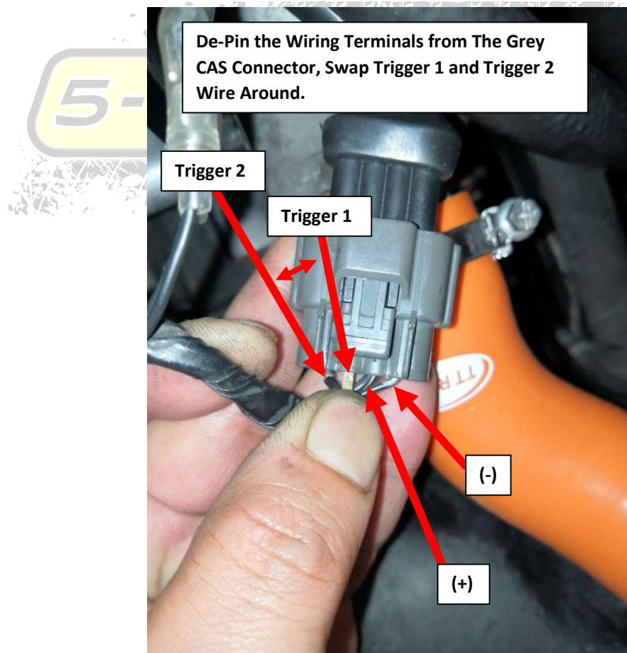
Figure 19 - Swapping Trigger Wires Around (Required on Some ECUs)
