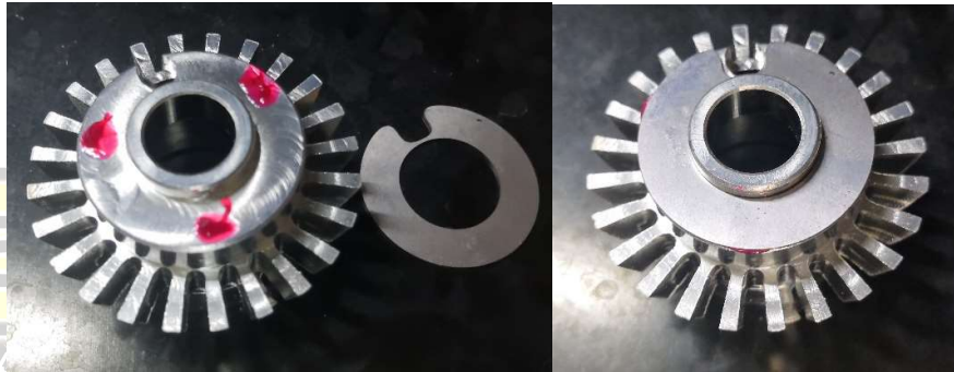
Figure 8 - Install Shim onto Trigger Wheel to reduce the Gap ONLY IF REQUIRED .
