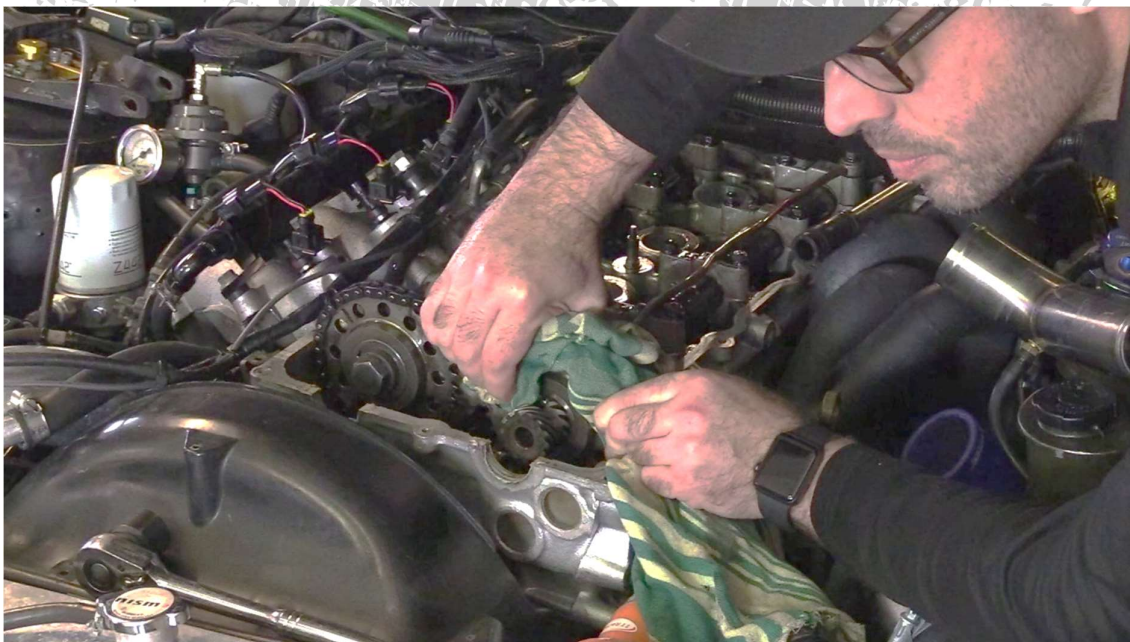
Figure 4 - Remove the Exhaust Cam Sprocket Bolt
