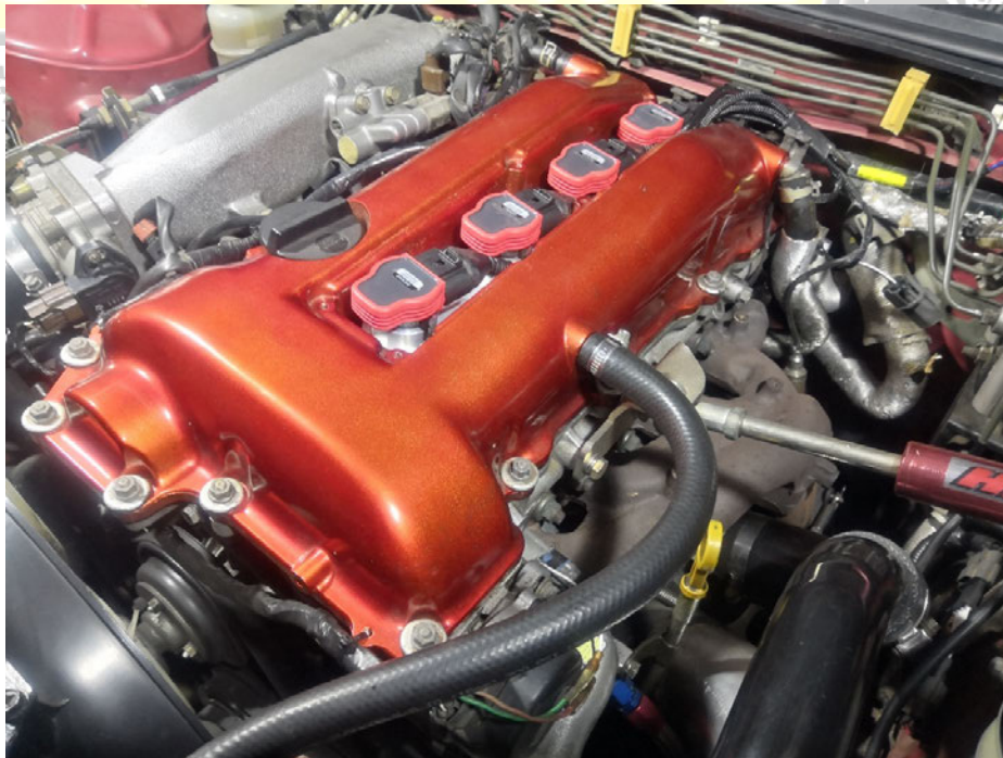
Figure 3- Tidy up the Harness and Seat the Coils
