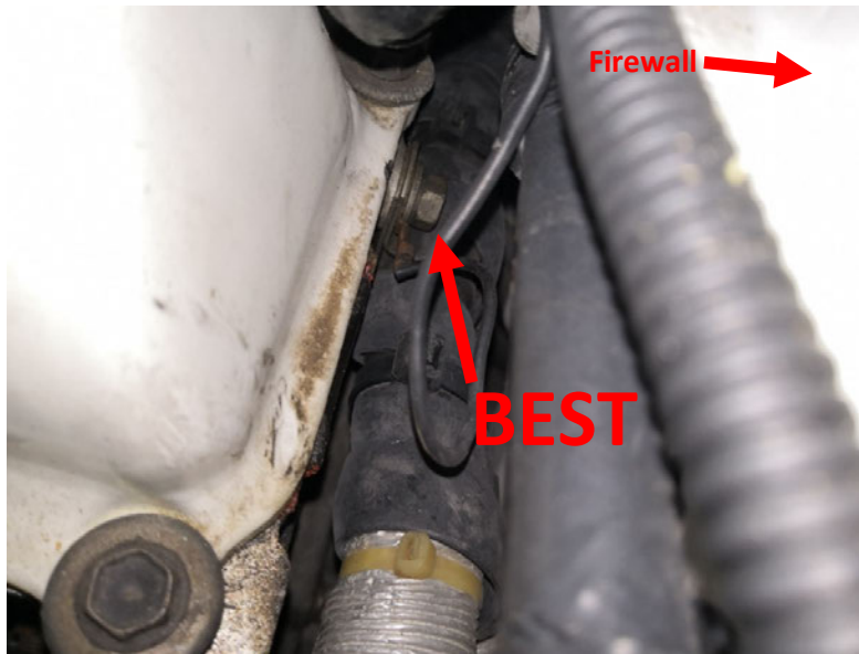
Figure 5 – Bolt down the other ground wire ring on stock ground position behind the head
