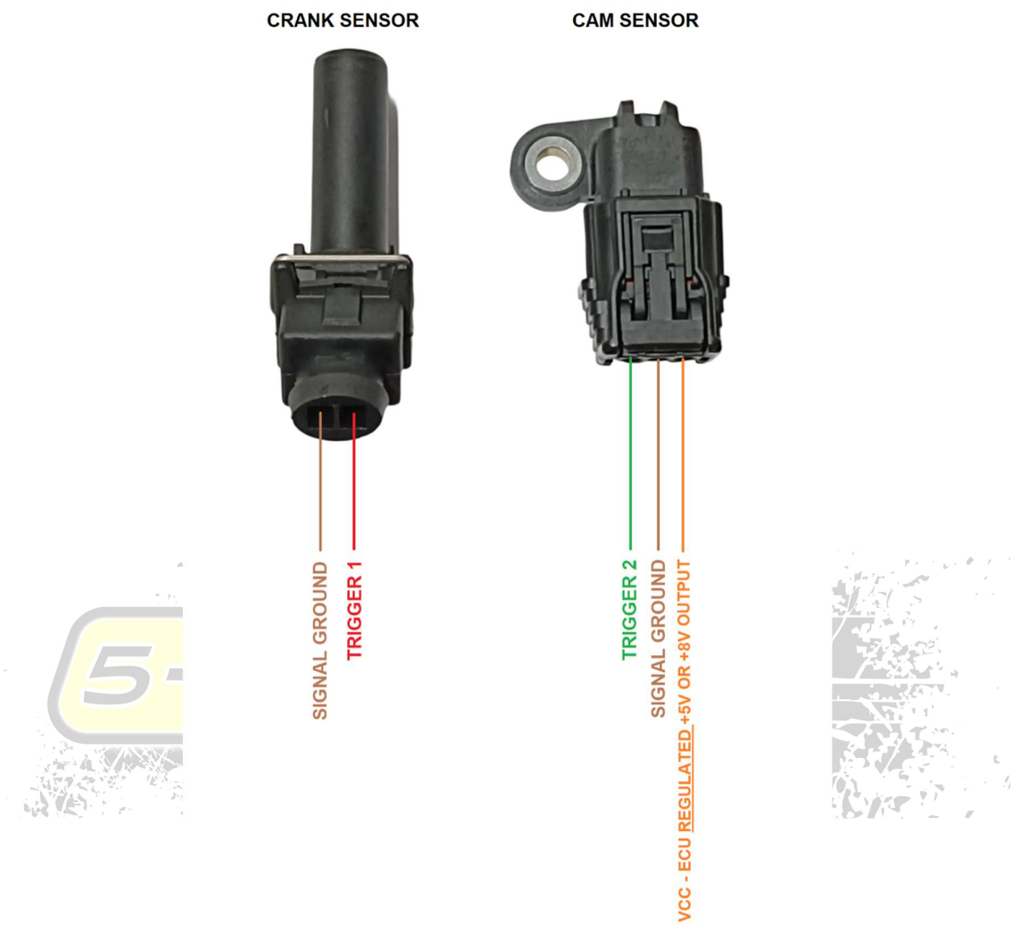
Figure 11 – 5-0 Ignite Race Series RB Trigger Sensor Pinout
