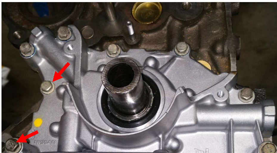
Figure 1 - Remove indicated bolts on the oil pump
