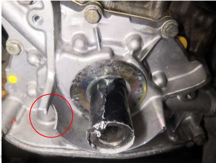
Figure 2 - Grind slot on oil pump housing
