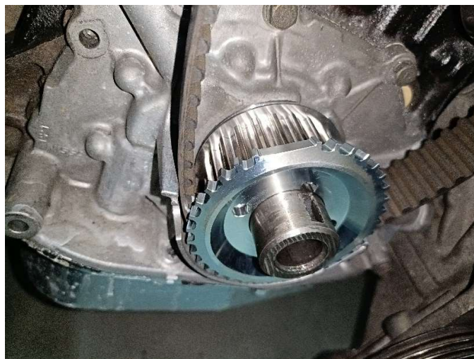
Figure 3 - Install your timing belt prior to sliding your sprocket in
