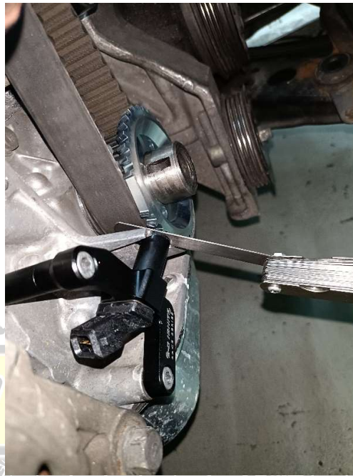
Figure 4 - Setting sensor gap
