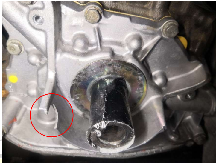
Figure 2 - Grind slot on oil pump housing
