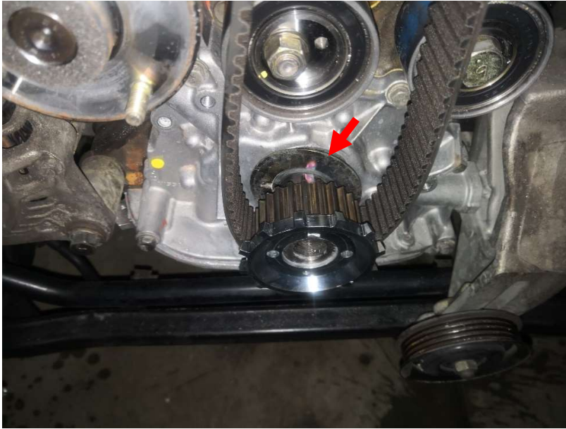
Figure 3 - Sliding your Sprocket In
