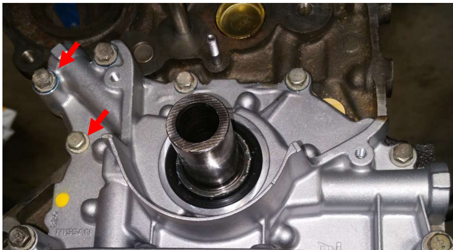
Figure 1 - Remove Bolts on Oil Pump
