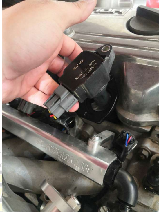
Figure 4 – Plug the connector onto the coil before completely mounting the coil onto the bracket
