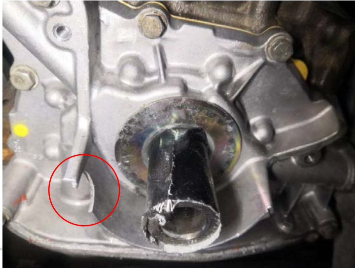
Figure 2 - Grind Slot on Oil Pump Housing
