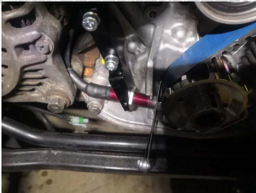
Figure 4 - Setting Sensor Gap
