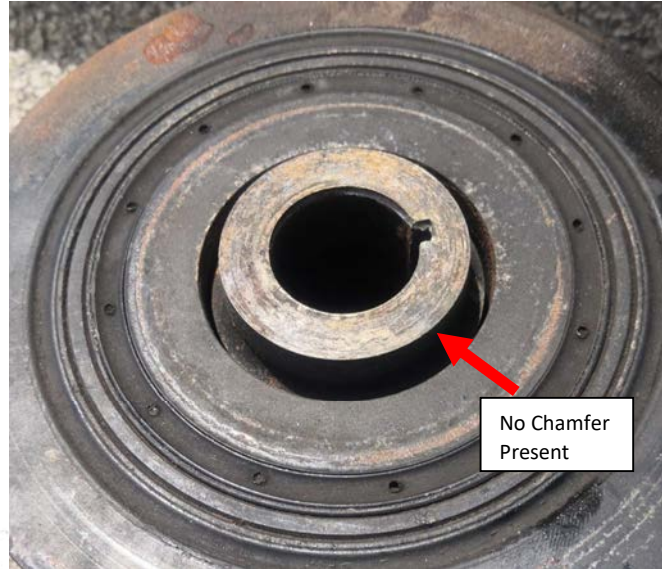
Figure 14 - R32 GTR OEM Crank Pulley 'A' (Insufficient Chamfer)
