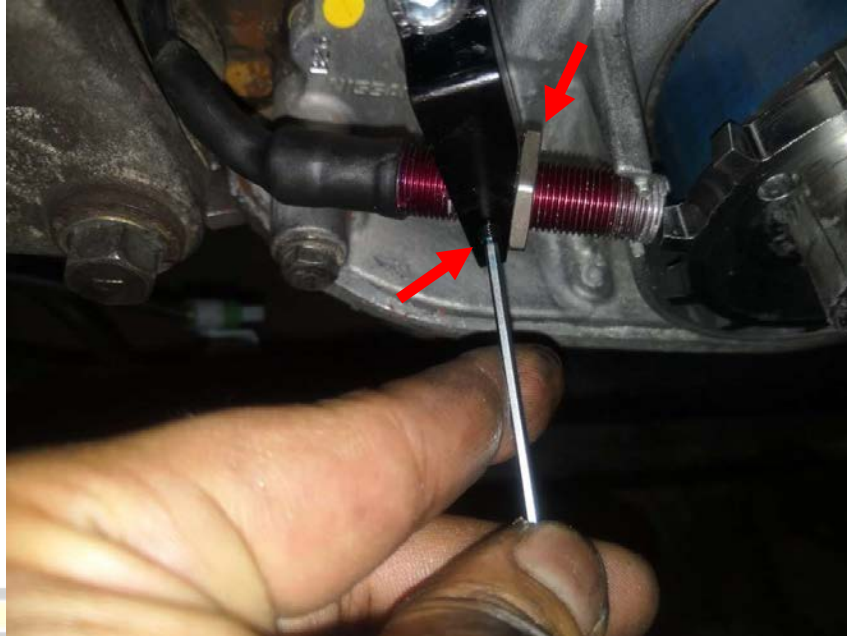
Figure 5 - Locking the Sensor into Place
