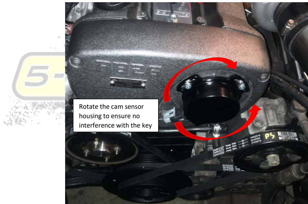
Figure 12 - Cam Sensor Clearance Check
