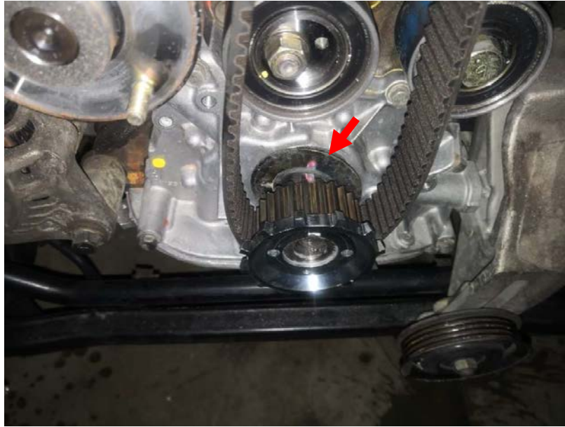
Figure 3 - Sliding your Sprocket In
