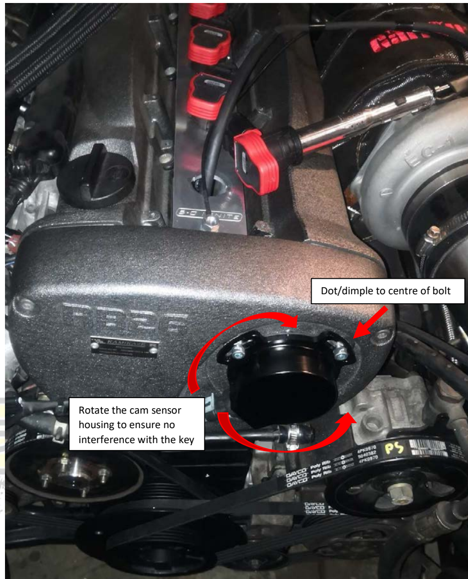
Figure 7 - Cam Sensor Housing Position
