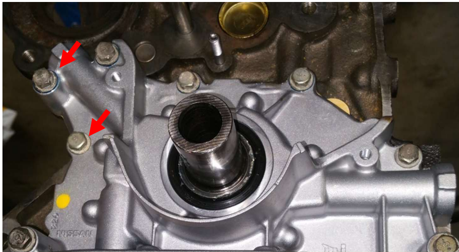
Figure 1 - Remove Bolts on Oil Pump
