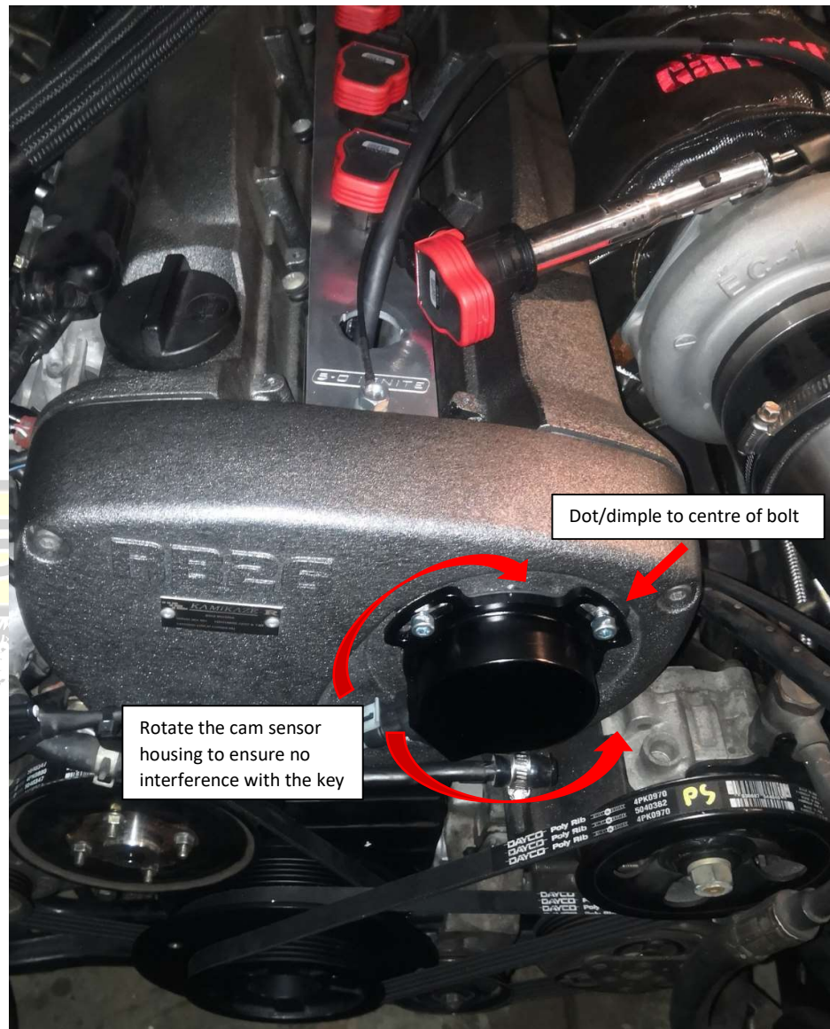
Figure 7 - Cam Sensor Housing Position
