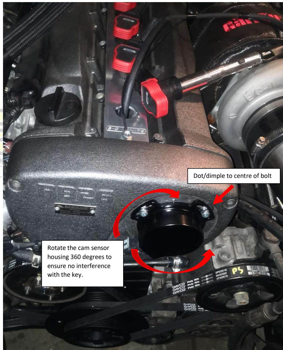
Figure 7 - Cam Sensor Housing Position (cam sensor housing old version shown)
