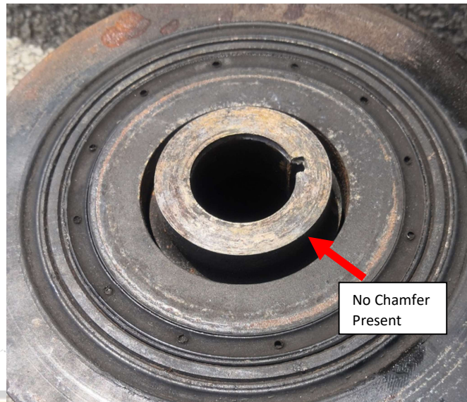
Figure 13 - R32 GTR OEM Crank Pulley 'A' (Insufficient Chamfer)
