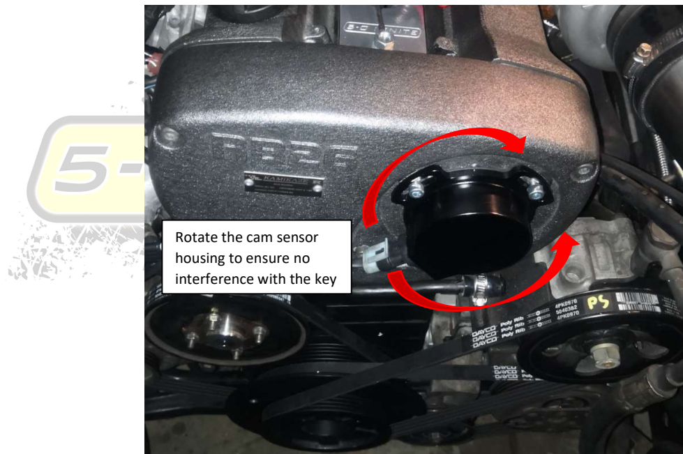
Figure 11 - Cam Sensor Clearance Check
