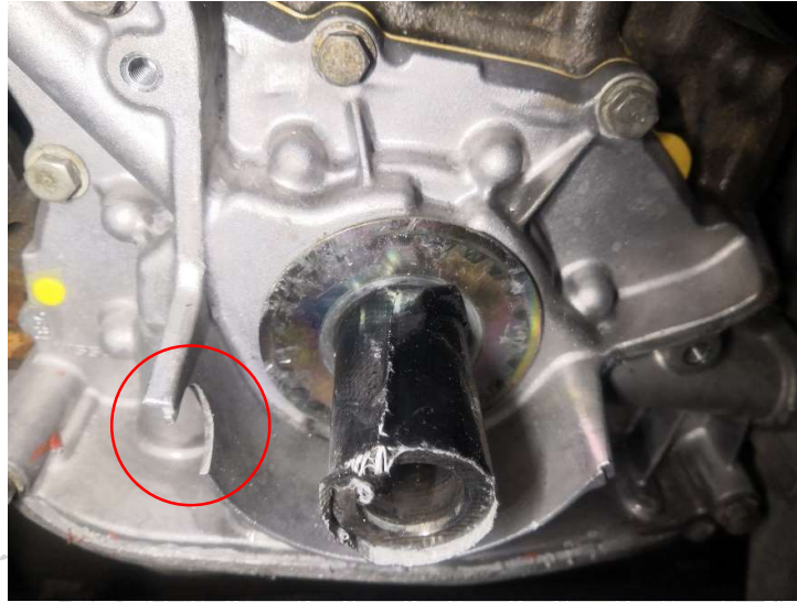
Figure 2 - Grind Slot on Oil Pump Housing
