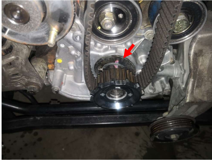
Figure 3 - Sliding your Sprocket In (photo shown with 12 tooth version)
