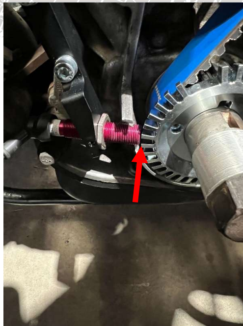
Figure 4 - Setting Sensor Gap
