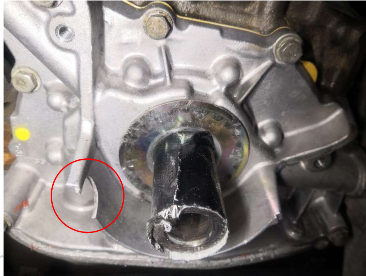
Figure 2 - Grind Slot on Oil Pump Housing
