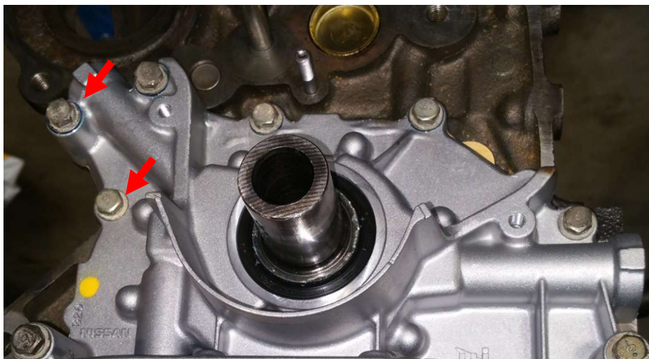
Figure 1 - Remove Bolts on Oil Pump
