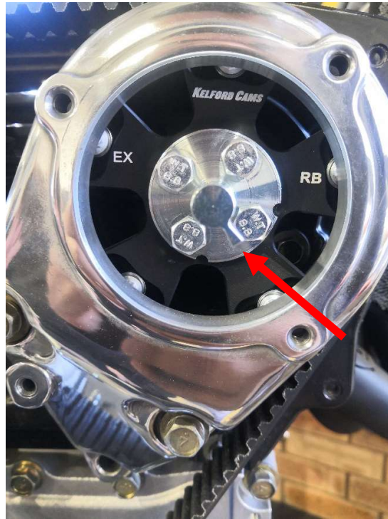
Figure 6 - Position of Cam Key when Engine at TDC
