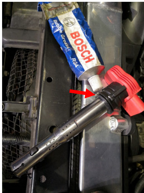
Figure 10 - Apply rubber grease to the lip of the ignition coils
