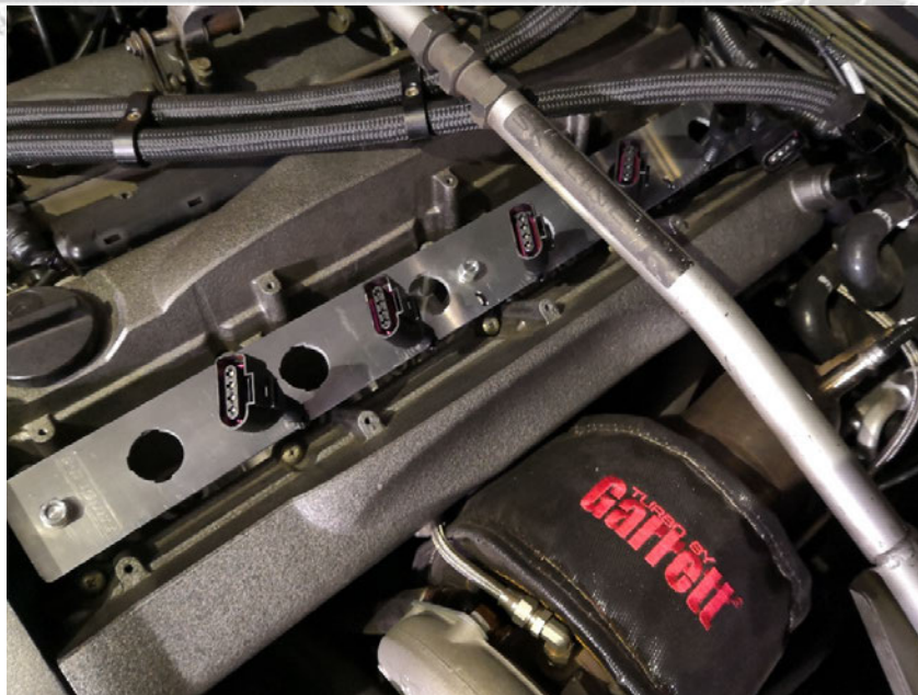
Figure 8 - Assembly of harness and mounting plate to the engine
