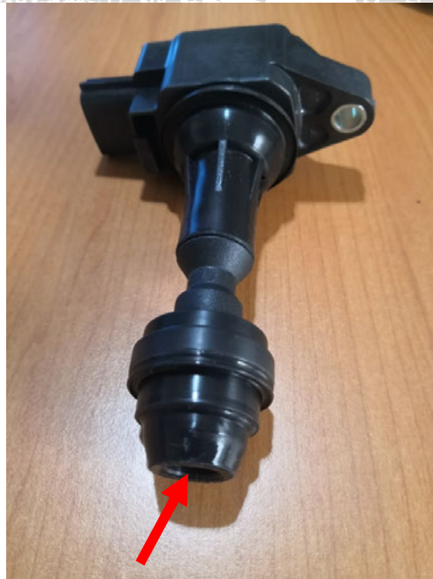
Figure 3 – Apply Di-Electric Grease on the Inside of the Stalk Tip
