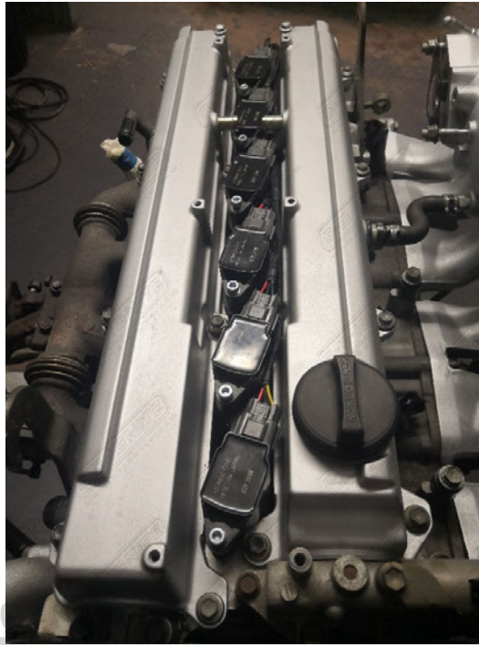
Figure 6 - Tighten the Coils onto the Mounting Bracket
