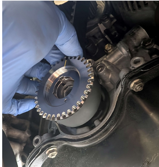
Figure 2 – Install crank sprocket and slip timing belt into position before fully seating it home
