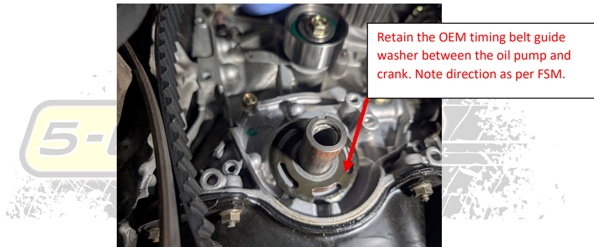
Figure 1 - Remove existing timing belt and sprocket
