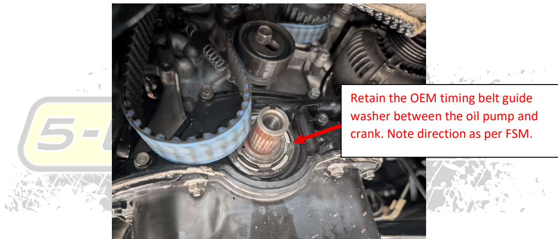
Figure 1 - Remove existing timing belt and sprocket
