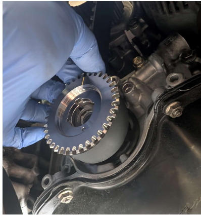
Figure 2 – Install crank sprocket and slip timing belt into position before fully seating it home (OBD2 oil pump shown)
