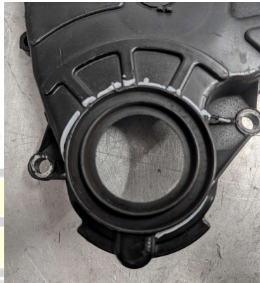
Figure 6 - Lower timing cover cut line
