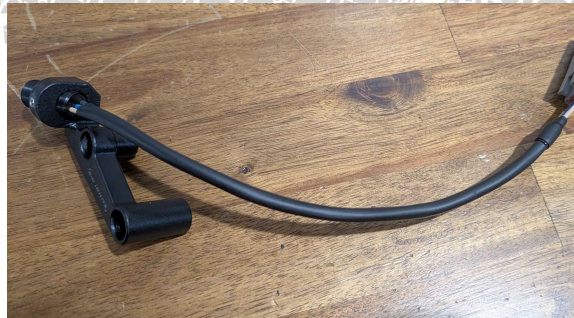
Figure 5 - Prepare the crank sensor wiring harness
