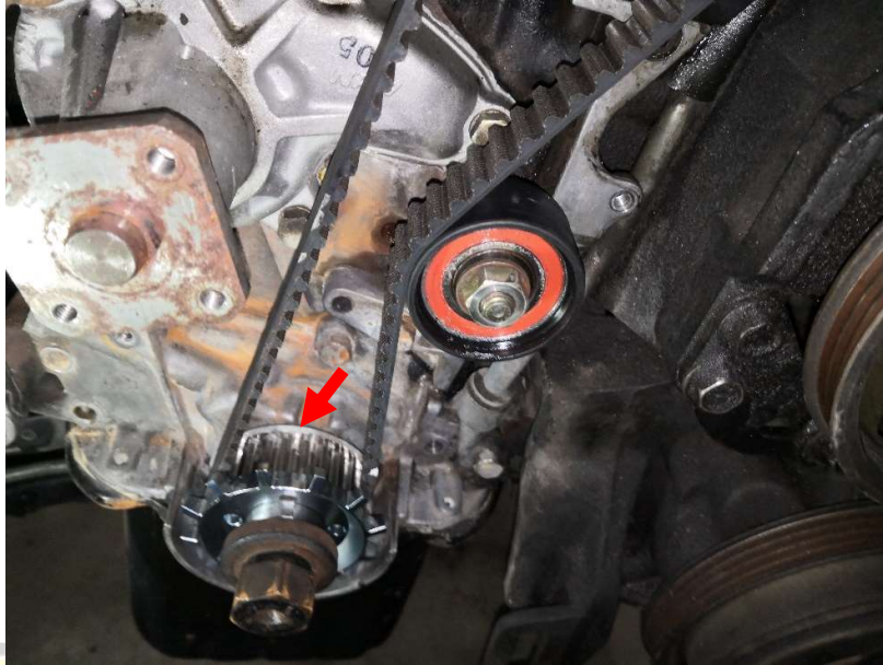
Figure 4 - Sliding your Sprocket In, Rear Backing Plate Installed
