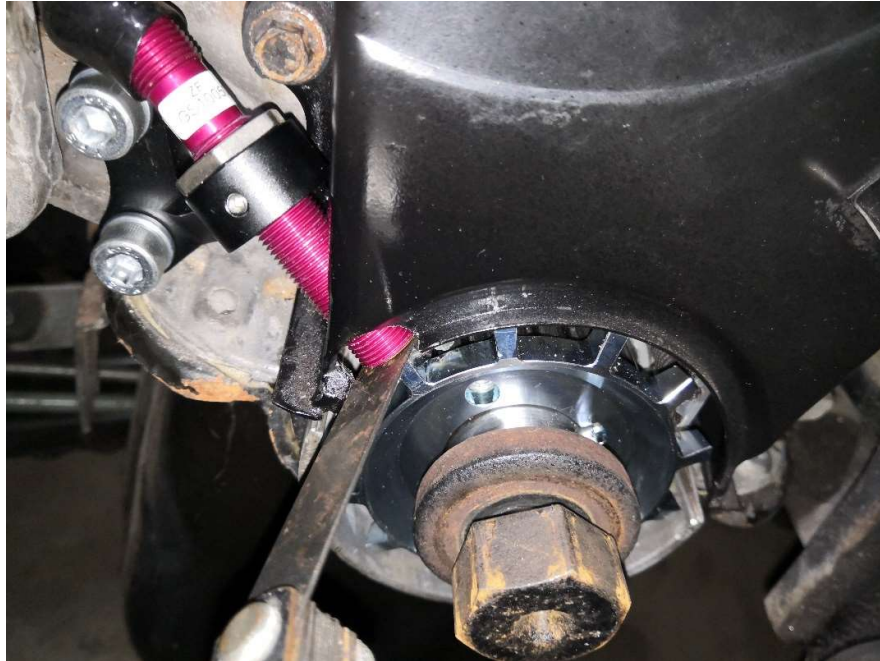
Figure 5 - Setting Sensor Gap
