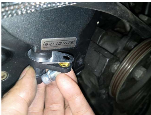
Figure 7 - Measure the Gap on The Cam Sensor
