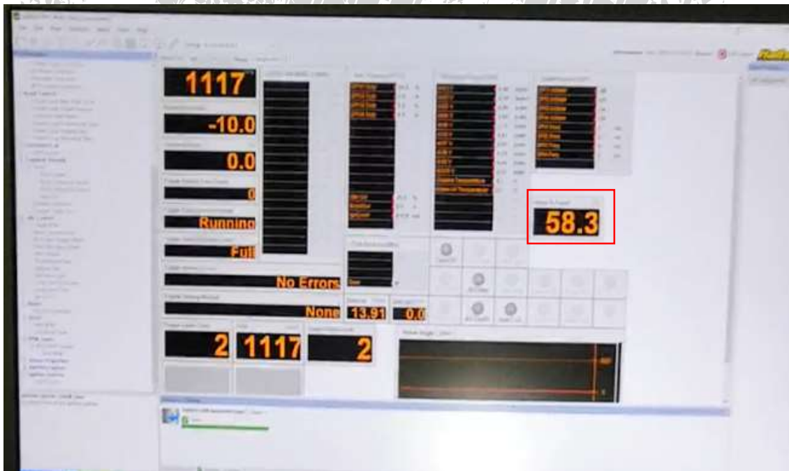
Figure 10 - Rotate the Cam Sensor Housing Until 'Home % Travel' displays ~50%
