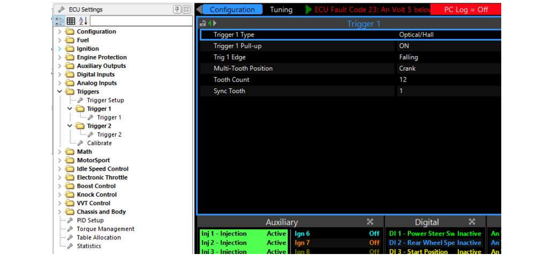
Figure 12 - Link G4X Trigger 1 Setup
