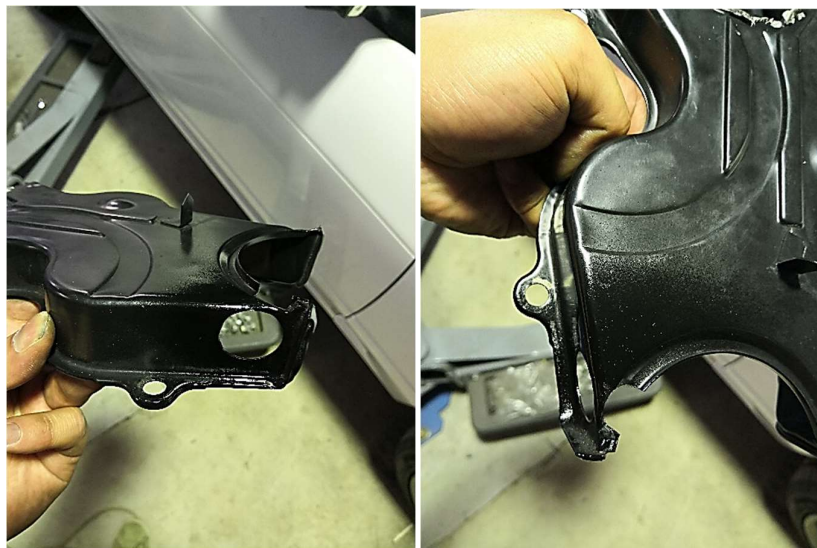
Figure 3 – Cut a Slot on The Lower Timing Cover for Crank Sensor Provision
