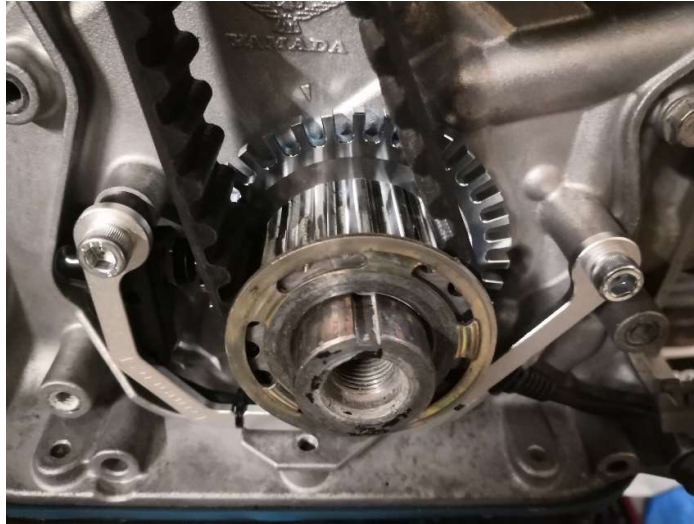
Figure 6 - Install the outer timing belt washer (note direction as per FSM)
