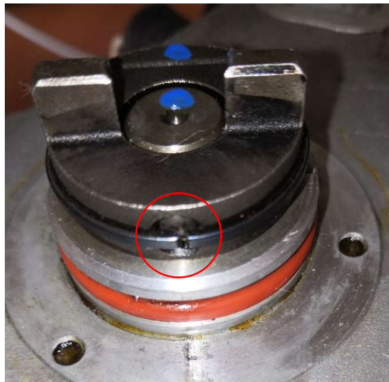
Figure 9 - Rotate c-clip to align with pin hole
