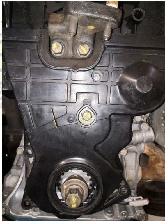
Figure 7 - Install the lower timing belt cover
