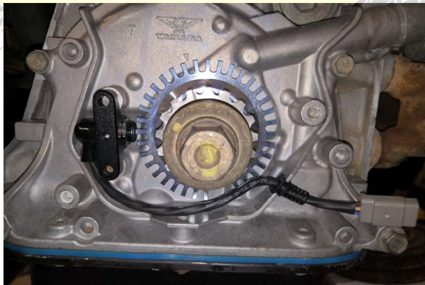
Figure 1 - Install the supplied crank sprocket and crank sensor
