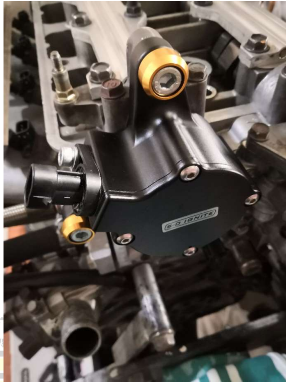
Figure 14 - Install the cam sensor unit onto the engine
