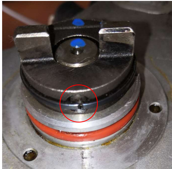
Figure 9 - Rotate c-clip to align with pin hole
