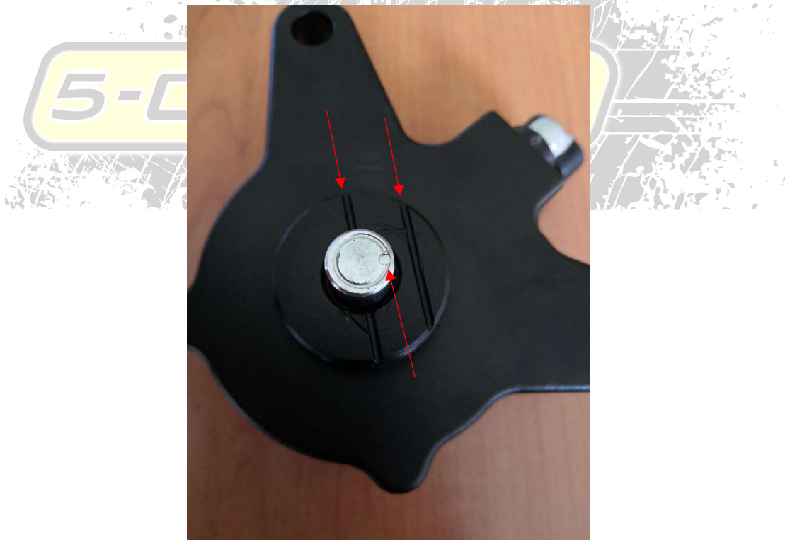
Figure 11 - Alignment marker on the shaft
