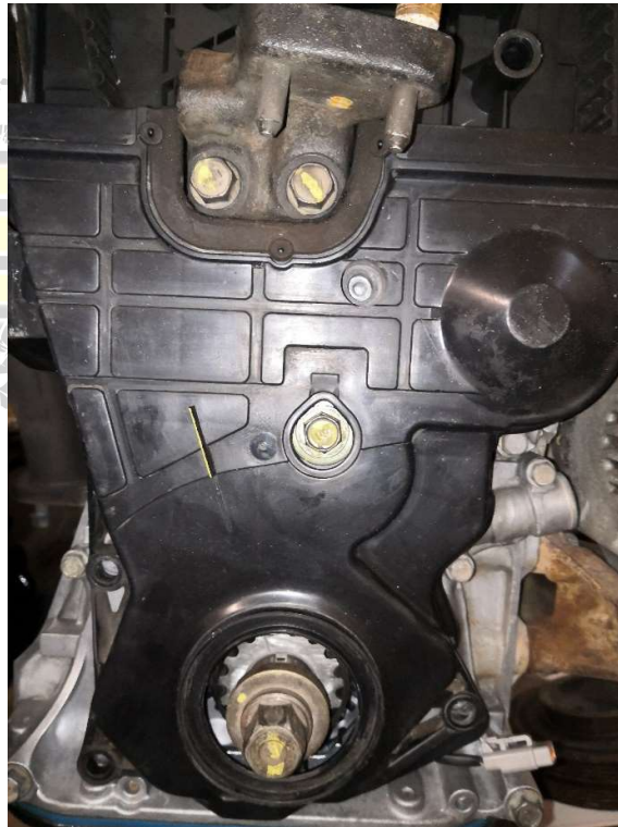
Figure 7 - Install the lower timing belt cover
