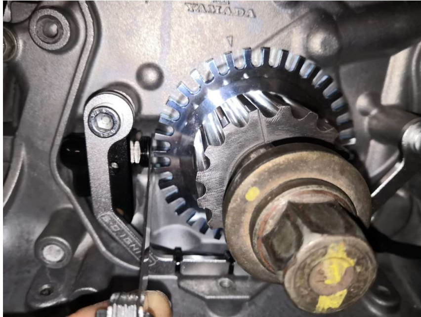
Figure 4 - Check the gap between the crank sensor and trigger tooth
