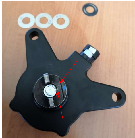
Figure 12 - Install the correct combination of shims behind the drive key (note the drive key alignment)
