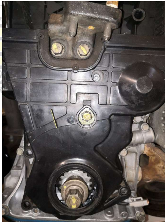
Figure 7 - Install the lower timing belt cover
