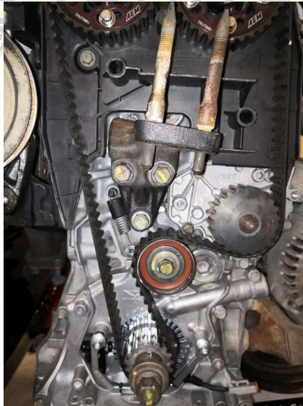
Figure 5 - Install the timing belt
