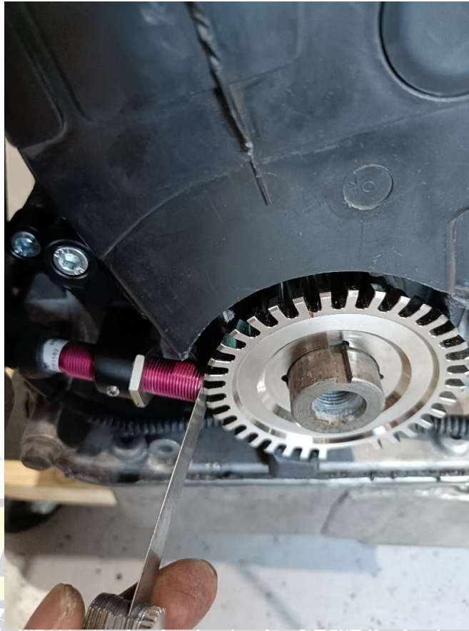
Figure 11 – Re-install the crank sensor
