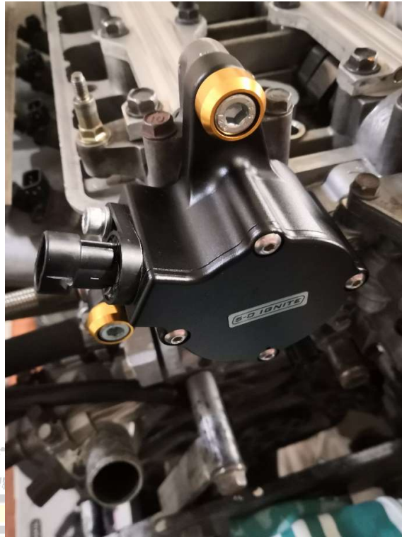
Figure 20 - Install the cam sensor unit onto the engine
