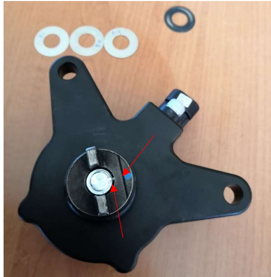
Figure 18 - Install the correct combination of shims behind the drive key (note the drive key alignment)
