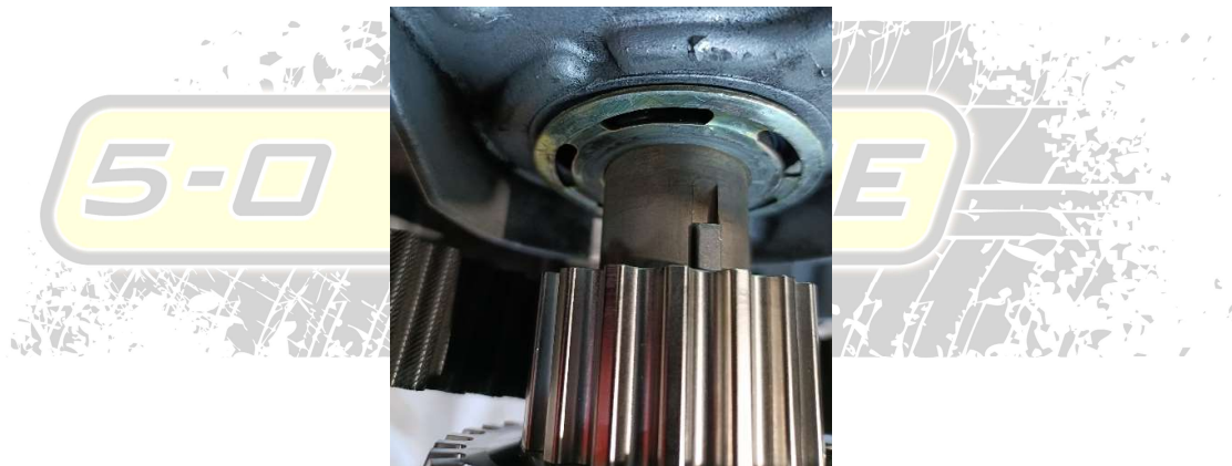
Figure 3 – Install crank sprocket and slip timing belt into position before fully seating it home
