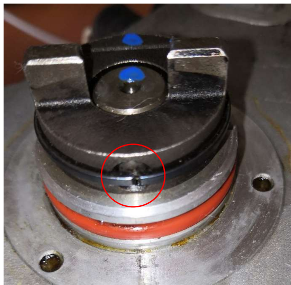
Figure 15 - Rotate c-clip to align with pin hole
