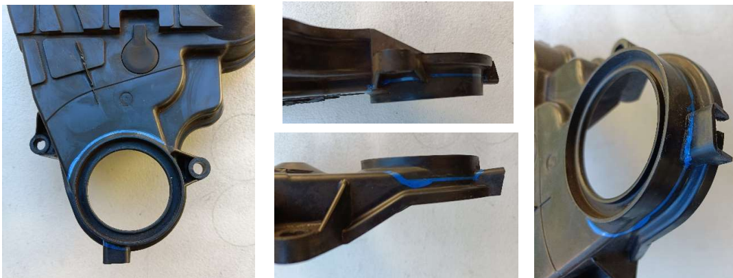
Figure 8 - Lower timing cover cut line
