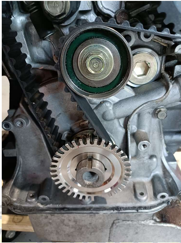
Figure 5 - Timing belt installed
