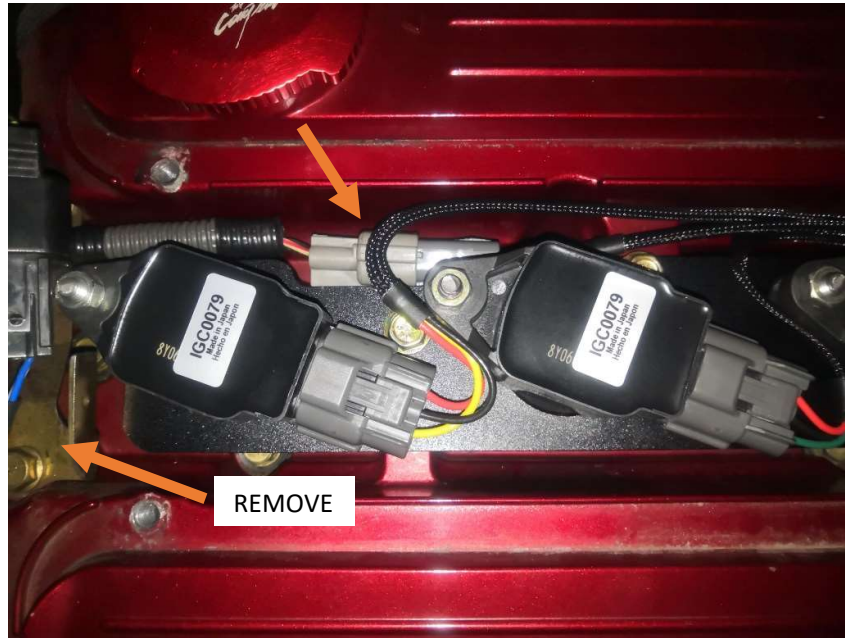
Figure 2 – Tucking the Connector and Removing Bracket
